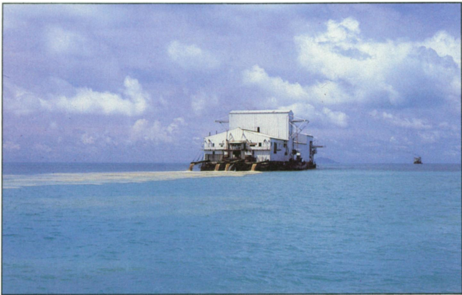
Bucket dredge operating in Phuket Bay at about 22-meters depth. This dredge has been in operation since the 1960s with a digging capacity of 320 000 m 2 · month -1 . Only a very small fraction is retained as tin ore (about 0.3 kg · m -3 of sediment). The rest is discharged as mine tailings which create the turbid plume. Most of the discharge settles in the vicinity of the dredge while lighter particles, especially fine sand and silt clay components, are dispersed by tidal currents. Another dredge can be seen at the horizon. Photo: H. Chansang.
